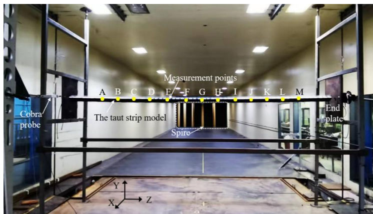
(a) Experiment setup of the taut-strip model
